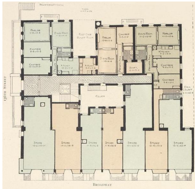
Image 10: Ground floor plan of the Saxon, showing Broadway storefronts: Source: NYPL Digital Archive.
